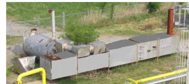
Duct Burner Test Rig at Zeeco. The simulated TEG is cooled by a running the TEG through a boiler to control the TEG inlet temperature to the duct runner at the correct temperature.
