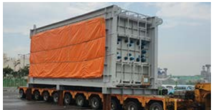
ZEECO Waste Heat Recovery Boiler
