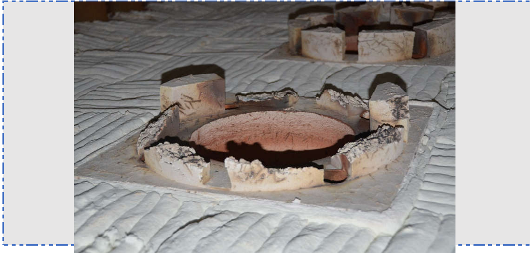
Burner 29 tile sections broken and missing.
