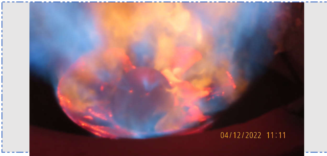
Burner 3 cone and coking build-up.
