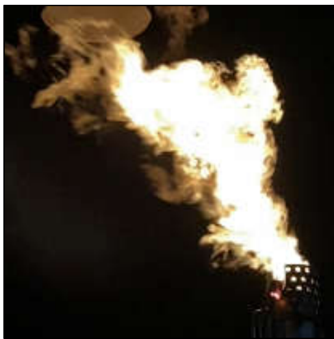
Figure 1. Low flow flaring 100% ammonia.
