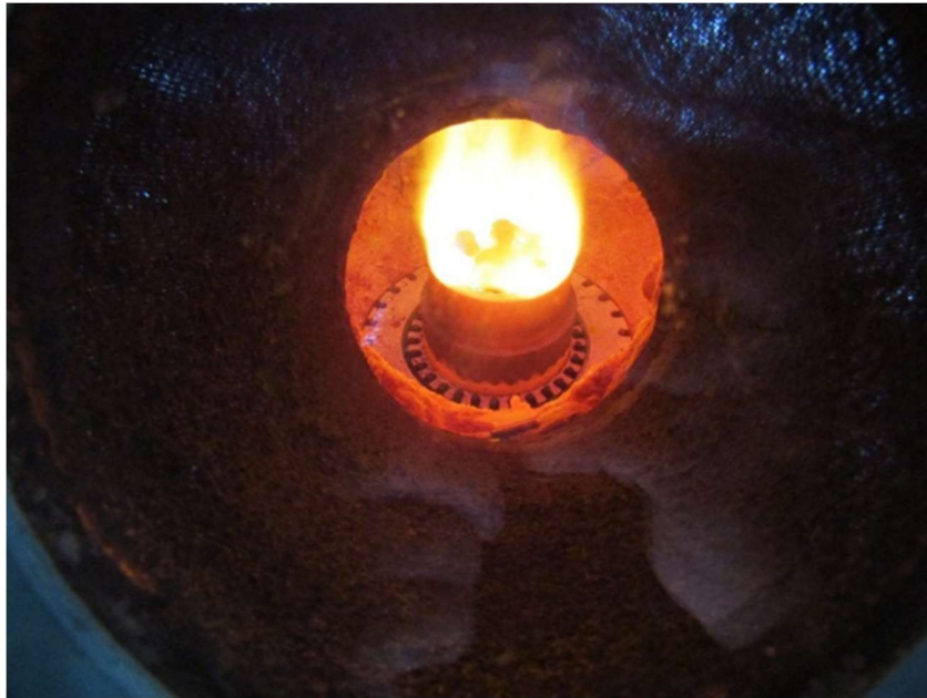
Figure 7. FREE JET firing 3.4 MM Btu/hr with 885F APH firing 100% ammonia.
