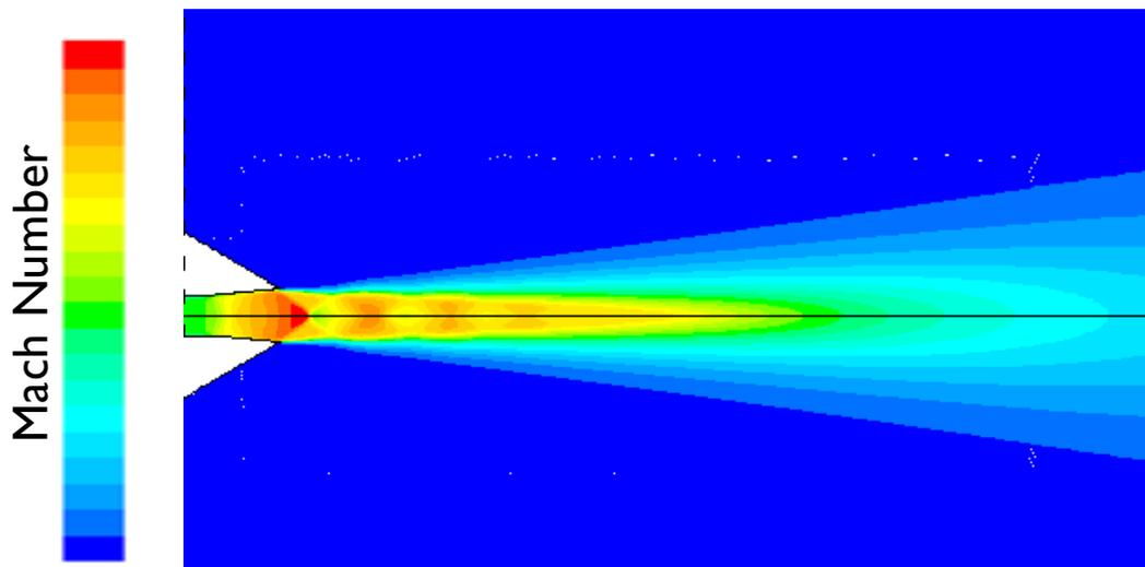
**Figure 8. Supersonic nozzle CFD velocity profile**
