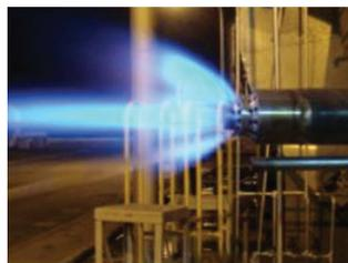
*ZEECO high-energy pilot burners are fully tested to ensure reliable, long-term operation in severe service, and can even be ignited and fired while completely submerged underwater.*
