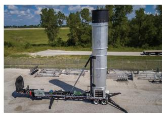
The Zeeco Zephyr trailer-mounted enclosed vapor combustor produces zero grade-level radiation, has full turndown capability, produces no smoke and has the ability to relieve inert waste streams by using an assist gas-injection system. (Source: Zeeco Inc.)
