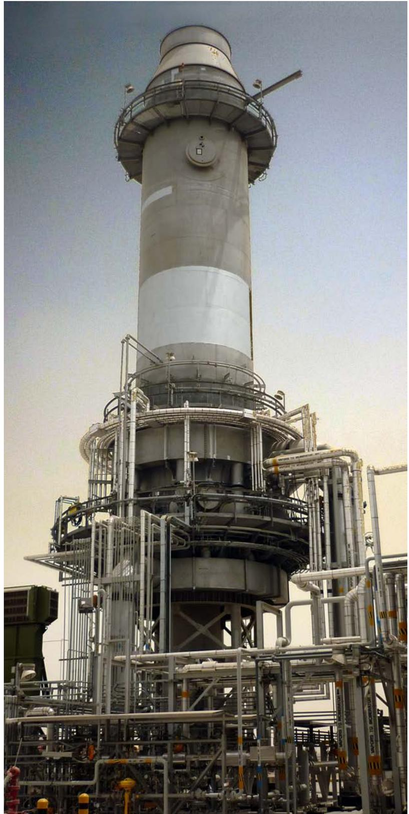
*ZEECO Nitrogen Bearing Waste Thermal Oxidizer*
