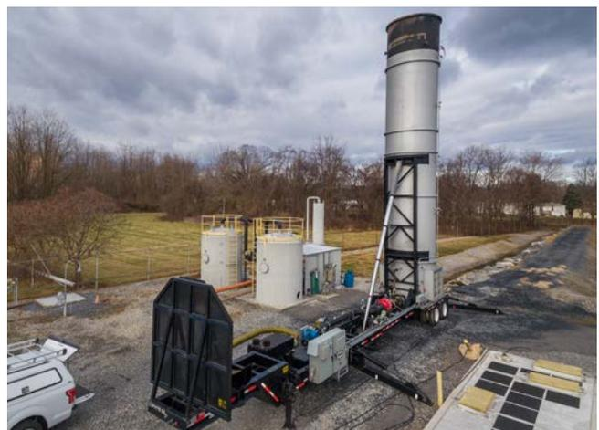
*Zeeco's Zephyr portable VCU*
