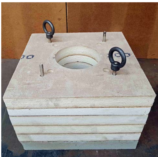
Figure 5. Side view of modular tile design showing attached eye bolts for manoeuvring tile into place.
