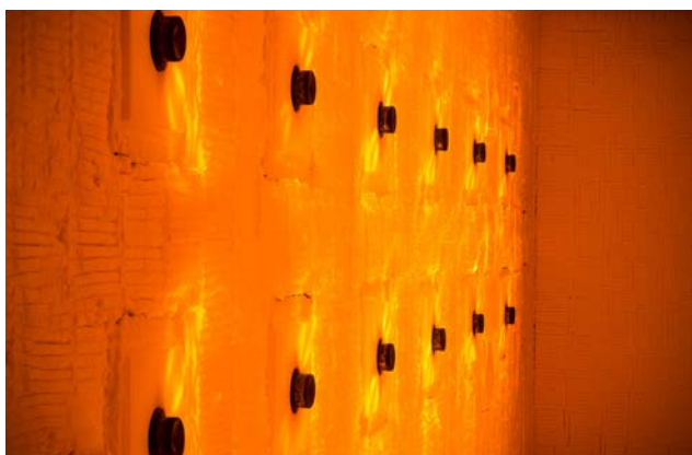
Figure 6. Operating radiant wall burners in furnace using Zeecolite tile.
