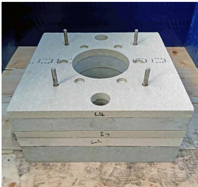
Figure 4. Side view of modular tile design showing ceramic fibre insulation boards and embedded anchor system.
