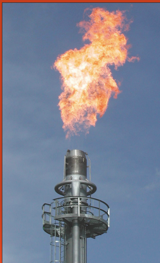
Figure 1 A Zeeco AF air assisted flare visually observed to be operating smokelessly at a proper air to fuel gas ratio.
