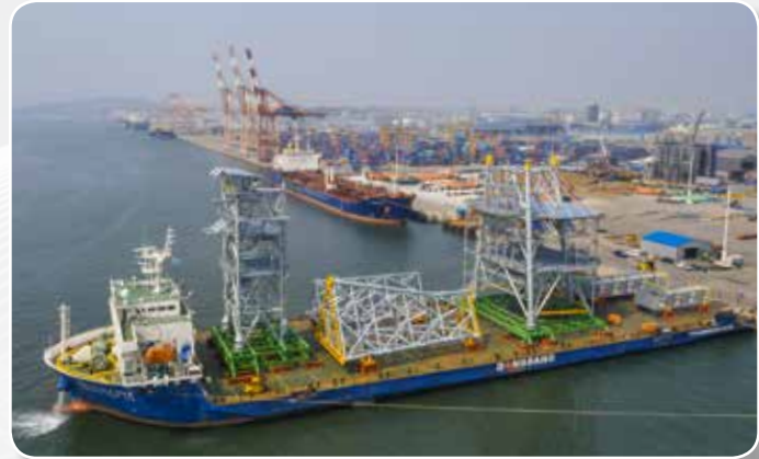
Modularized Flare Derrick Ready for Transport
